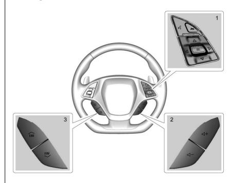
Some audio controls can be adjusted at the steering wheel.
