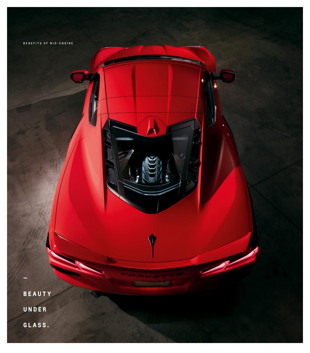
Your first impression is that beautiful engine behind the cockpit, visible on coupe models. Why is it located there? First, this puts the weight of the engine over the rear-driving wheels to enhance traction. With the engine behind the cockpit, there's more forward visibility. And with the seats positioned closer to the front wheels, the driver and passenger are at the car's center of gravity.
